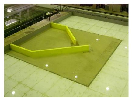
Figure 7. The harbor model used in the laboratory experiment. The size of the harbor was approximately 6.0 m by 6.0 m. The typical harbor shape was applied in this study.
