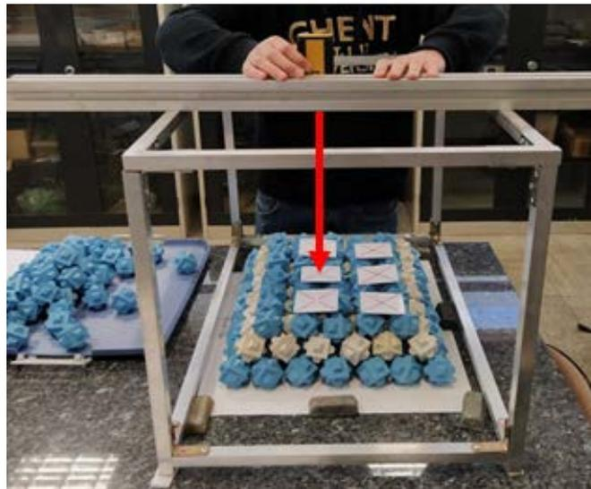
Figure 5. Measurement of layer thickness in the physical placement tests using a rectangular grid with  $a/D_n=1.40$  and  $b/D_n=1.30$  (Keyser and Jacobs, 2020)
