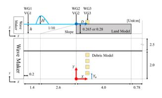
Figure 1 -Outline of experiment (h: water depth,  $Y_0$ : Initial distance in the Y direction from the reference point to the center of gravity of the drifting object)
