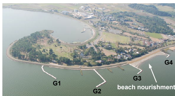
Figure 3. Experimental beach nourishment along with the construction of groins.
