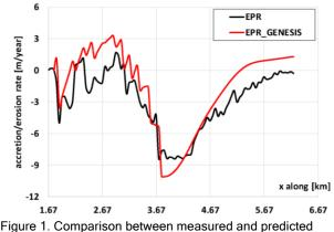
Figure 1. Comparison between measured and predicted EPR for the groins permeability P=0.2 and for the K=0.2.
