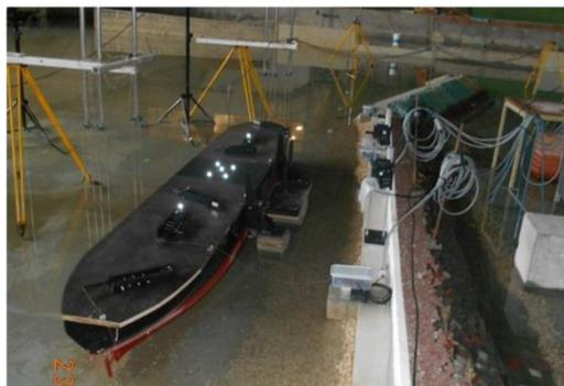
Figure 2 - Ship's model with moorings instruments and optical point trackers
