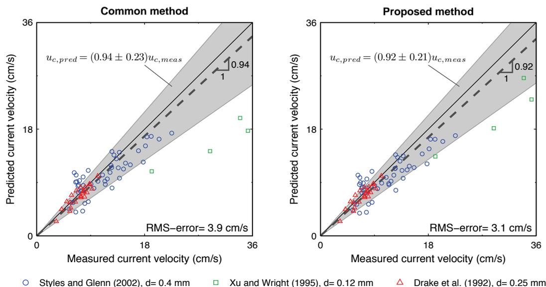
Figure 4. Comparison between predicted and measured current velocities 100 cmab. The solid line denotes perfect agreement while the dashed line shows the average slope of the data points and the gray band covers  $\pm 1$  standard deviation of the average slope, corresponding to an underprediction of  $6 \pm 23\%$  and  $8 \pm 21\%$ , respectively, for the common (left panel) and proposed (right panel) methods.
