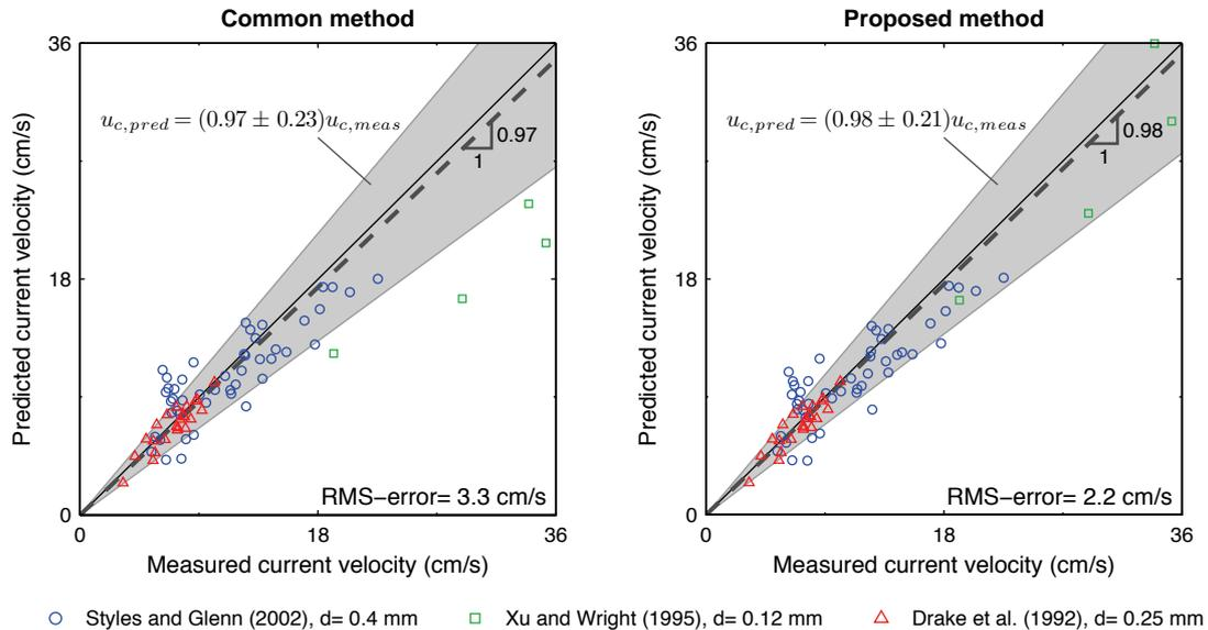
**Figure 5. Comparison between predicted and measured current velocities 100 cmab using the 1/10 near-bottom velocity in the Shields parameter. The solid line denotes perfect agreement while the dashed line shows the average slope and the gray band covers  $\pm 1$  standard deviation of the slope, corresponding to an underprediction of  $3\pm 23\%$  and  $2\pm 21\%$ , respectively, for the common and proposed methods.**
