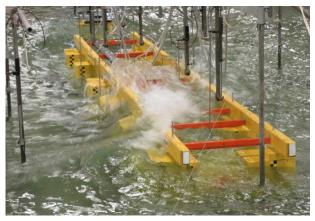
Figure 2 - Wave loads and pressures were measured on a 1/35 scale model of a gravity-based structure.
