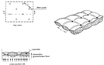
Figure 7, Principles of permeability of Filter Point Mattress
