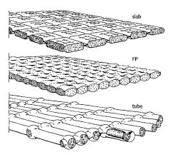
Figure 6 Examples of concrete-filled mattresses
