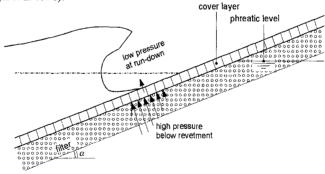
Figure 1, Pressure development in a revetment structure
