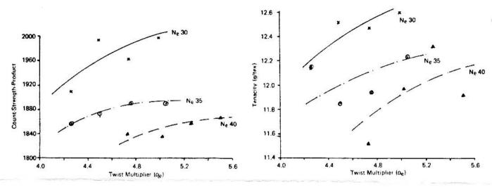
illustrating the influence of twist on the yarn strength (Count-Strength-Product and single yarn tenacity) in the case of Texas cotton and Figure 6 illustrating this influence in the case of California cotton.
