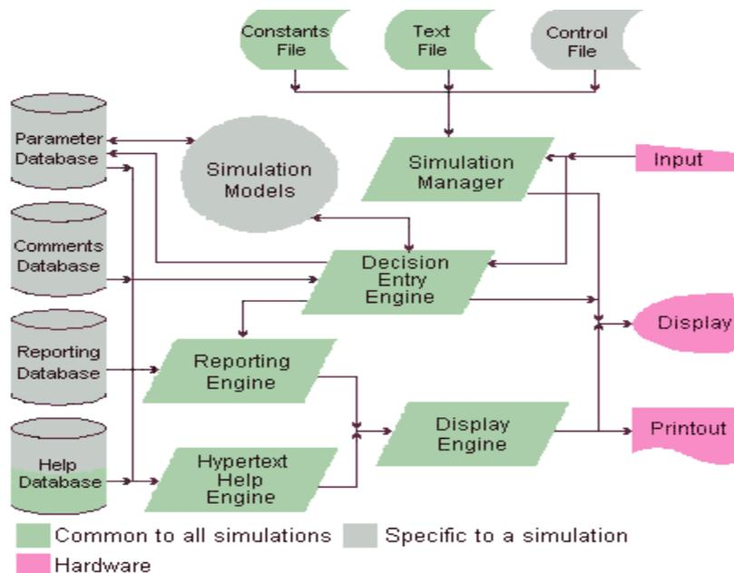
Figure 8: Software Architecture
