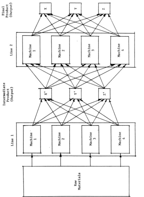
Figure 1 THE PROSIM MANUFACTURING PROCESS
