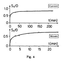
increased by a factor of 4 with respect to its undisturbed value, resulting in an increase in the sediment transport rate of a factor of 8. This explains why the scour below the pipe occurs so fast and so violently during the tunnel erosion.
