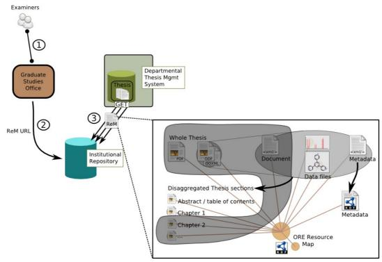
Illustration 14: The final stage - automated IR deposit
