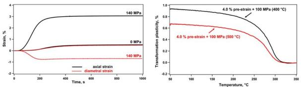
Figure 6 Evolution of axial and diametral strain during isothermal bainitic phase transformation at 340 °C following an austenitization at 1200 °C for 10 s with and without superimposed stress.
