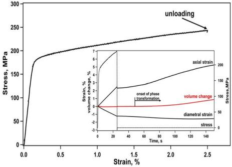
Figure 3: Stress-strain response of the supercooled austenite at 340 °C following an austenitization treatment at 1200 °C for 10 s. The chosen nominal strain rate was  $1 \times 10^{-3} \text{ s}^{-1}$ . In order to avoid the onset of transformation during tensile testing, the specimen was unloaded at 2.5 % total strain.
