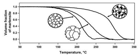
Figure 5: Influence of the prior austenitization treatment on the martensitic phase transformation behavior, data recompiled from [Lambers et al. 2010]. Austenitization treatments at 880 °C for 5min, 1050 °C for 60 s and 1200 °C for 10 s resulted in small austenite grains with residual carbides (indicated as black ellipsoids), small austenite grains without carbides and large austenite grain sizes, respectively.
