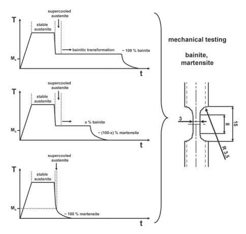
Figure 2: Schematic illustration of the cooling conditions considered in the present study, resulting in pure bainitic (a), pure martensitic (c) or a mixture of both microstructures (b) at RT. For the subsequent tensile test the cross-section in the gage section was reduced in order to guarantee for a failure within this regime.
