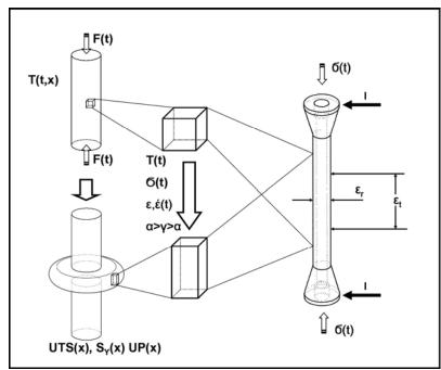
Figure 1: The thermo-mechanical coupled forging process investigated is influenced by several parameters such as strain  $(\varepsilon)$ , strain rate  $(\dot{\varepsilon})$ , temperature (T), and stress  $(\sigma)$ , which can all vary with time (t) and location within the work piece. Thin-walled hollow specimens were used in order to simulate the local temperature-time-deformation path of selected volume elements in the work piece, schematic recompiled from [Maier et al. 2009].
