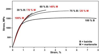
Figure 8: Stress-strain response of 51CrV4 steel in different microstructural states. The different volume fractions of bainite were formed isothermally at 340 °C following an austenitization treatment at 880 °C for 5 min.
