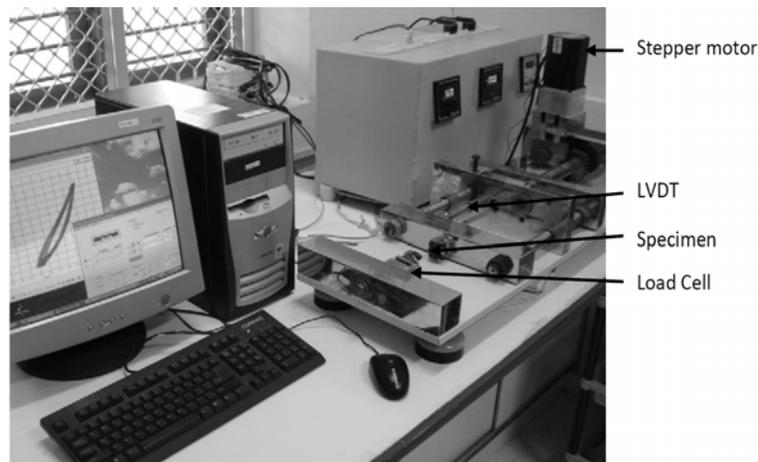
Figure 3 Experimental Set-up for Cyclic Loading Experiments on SMA Wires
