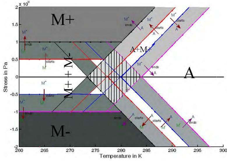
Figure 4: Non-zero dissipation ( $\bar{k}_1, \bar{k}_2, \bar{k}_3 > 0$ ) with linear hardening ( $\beta^{\epsilon^t}, \beta^\alpha > 0$ ): Phase Diagram. The shaded regions show the existence of pure phase (darker shades) or mixtures (lighter shades). The hashed region is the region of existence of all the three species.
