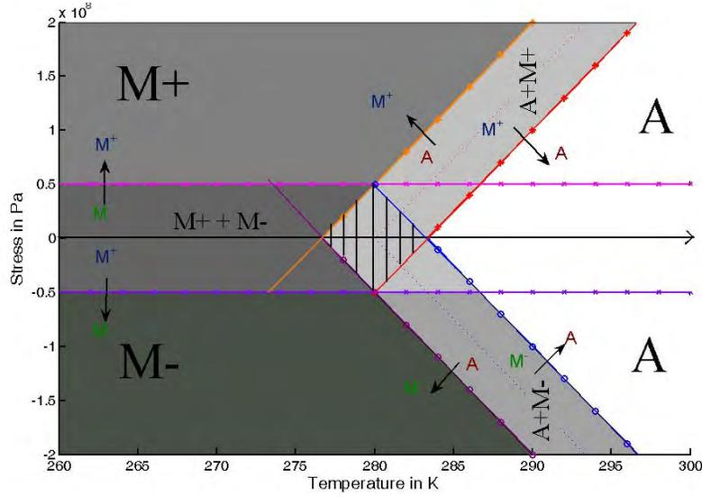
Figure 3: Non-zero dissipation ( $\bar{k}_1, \bar{k}_2, \bar{k}_3 > 0$ ) without hardening ( $\beta^{\epsilon^t} = \beta^\alpha = 0$ ): Phase Diagram. The shaded regions show the existence of pure phase (darker shades) or mixtures (lighter shades). The hashed region is the region of existence of all the three species.
