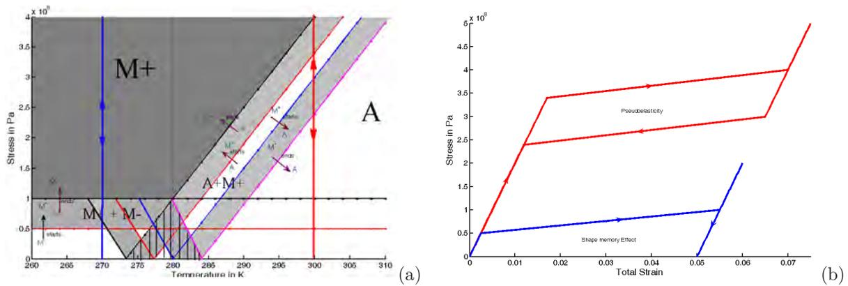
Figure 5: Isothermal loading. (a)Phase diagram for tensile loading, (b) Stress - Total strain plot. The shaded regions indicate existence of either a pure phase (darker shade or white) or mixed phases (lighter shade). The part that corresponds to the coexistence of all the three species is hashed here.
