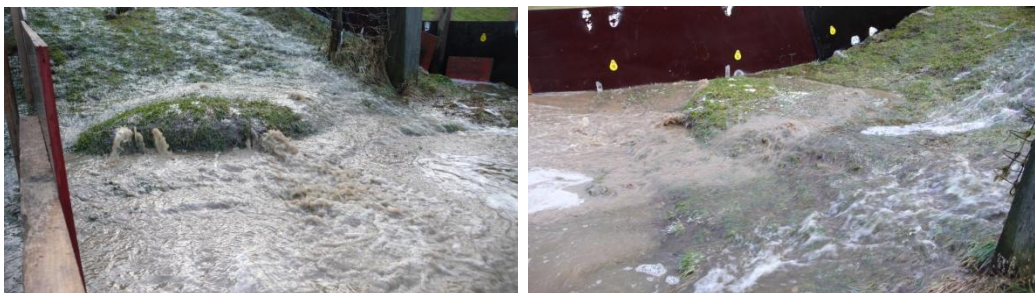
Figure 12. "Bulge out" mechanism before and after the water has flown out
