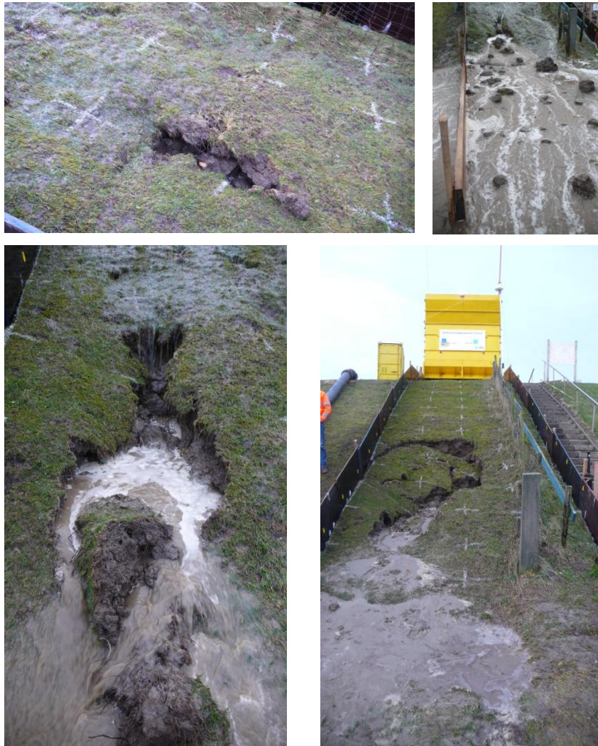
Figure 13. Consequent steps leading from “bulge out” mechanism to failure of slope section 3
