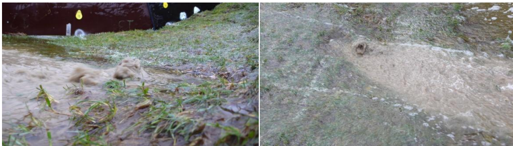
Figure 11. Sand containing well through tunnel of mole
