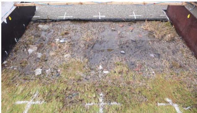
Figure 6. Final result of overtopping test section 1; various damaged locations (photo taken from the slope down)
