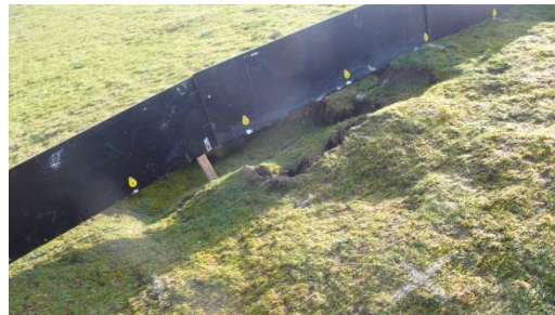
Figure 16 .Left: Water and sand flushing out tunnel of mole. Right subsidence of slope
