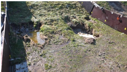
Figure 15. Damage at toe up to core of the dike, section 4
