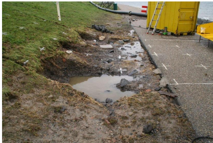
Figure 21. Final damage after the pilot run-up test.
