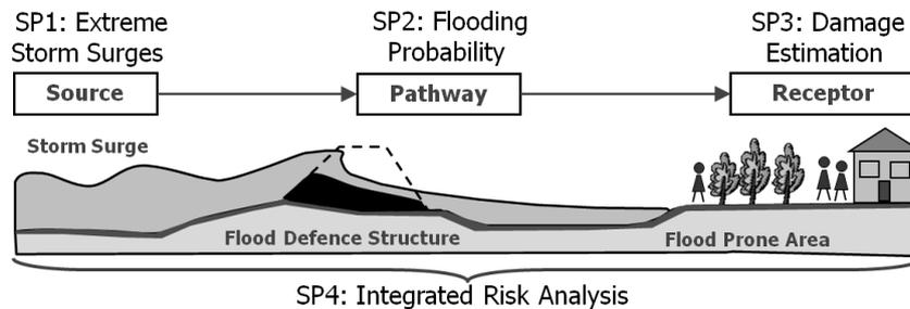
**Figure 1. Risk Source-Pathway-Receptor concept and subprojects (SP) as applied in XtremRisK.**
