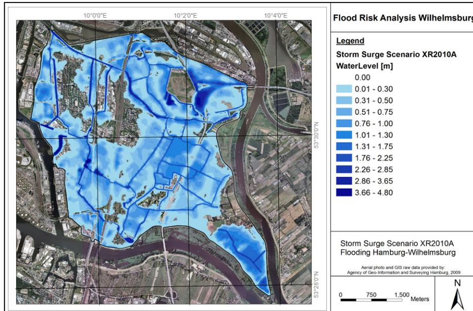
Figure 3. Flood depth for the XR2010A scenario in Hamburg-Wilhelmsburg visualized in a 10 m grid.
