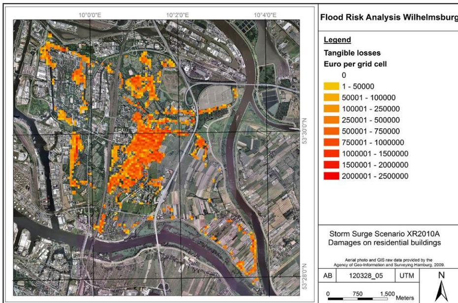
Figure 8. Tangible losses on residential buildings in Hamburg-Wilhelmsburg based on a 50 m grid.
