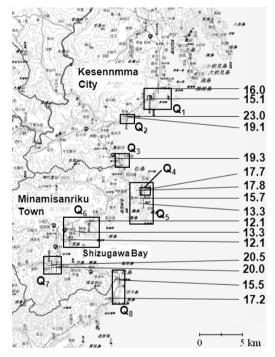
Figure 5. Distribution of inundation height measured by the authors in both the south of Kesennuma City and Minamisanriku Town (unit: m).
