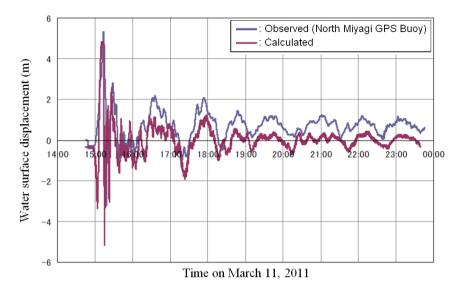
Fig. 11. Numerical result of water surface displacement at the position of North Miyagi GPS Buoy in comparison with the observed data through the GPS buoy (Kawai et al., 2011).
