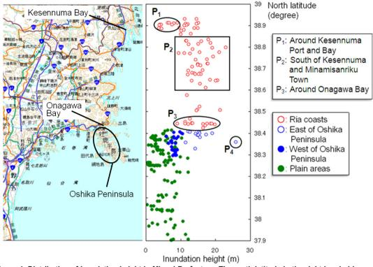
Figure 4. Distribution of inundation height in Miyagi Prefecture. The north latitude in the right-hand side graph corresponds to that in the left-hand side map. The data include a part of the trace survey results obtained by other teams of the JSG (Mori et al, 2012).
