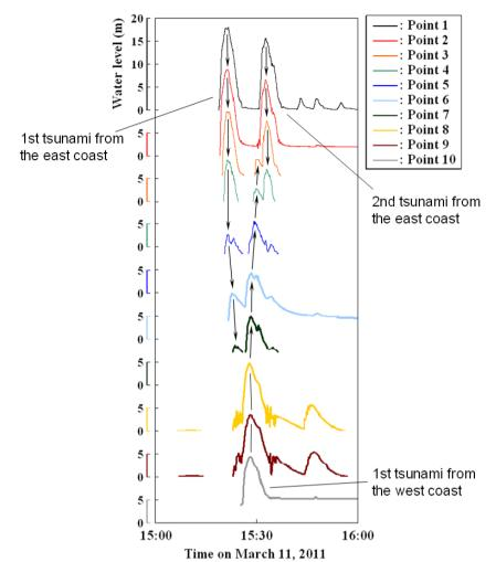
Fig. 13. Numerical result of time variation in water level at each point indicated in Fig. 12.
