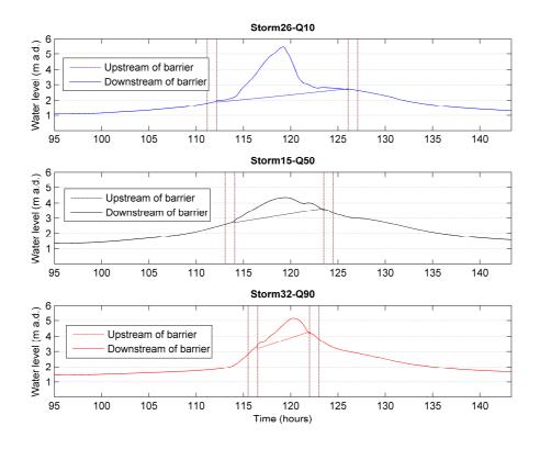
Figure 4. Water level variation during storm conditions upstream and downstream of the barrier for three storm-discharge combinations.
