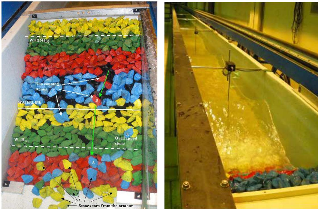
Figure 4 : Photograph of the Damaged Breakwater with Explanation of the Damage Calculation (left) and the Test Channel (right)
