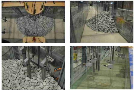
Figure 5. Breakwater roundhead in the flume after construction. Bottom right: undisturbed wave tests without structure but with instruments at the same positions as in the tests with structure.
