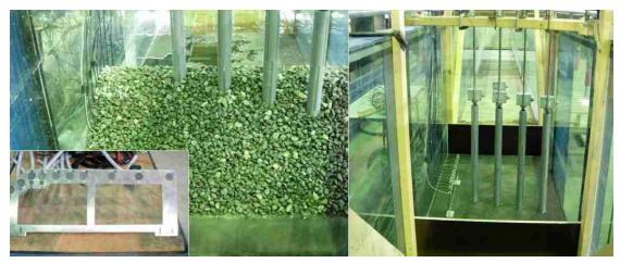
Figure 8. Experimental setup in the flume. The mount with pressure sensors is shown on the left; the array with wave gauges is shown on the right; the centre image shows the complete structure.
