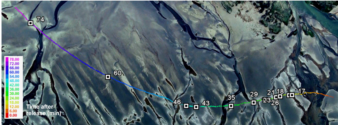
Figure 8: Drifter track from second release plotted on a Google Earth image taken 1 May 2009. Colours indicate the time after release. Squares indicate events with high backscatter, numbers give the associated time after release in minutes.
