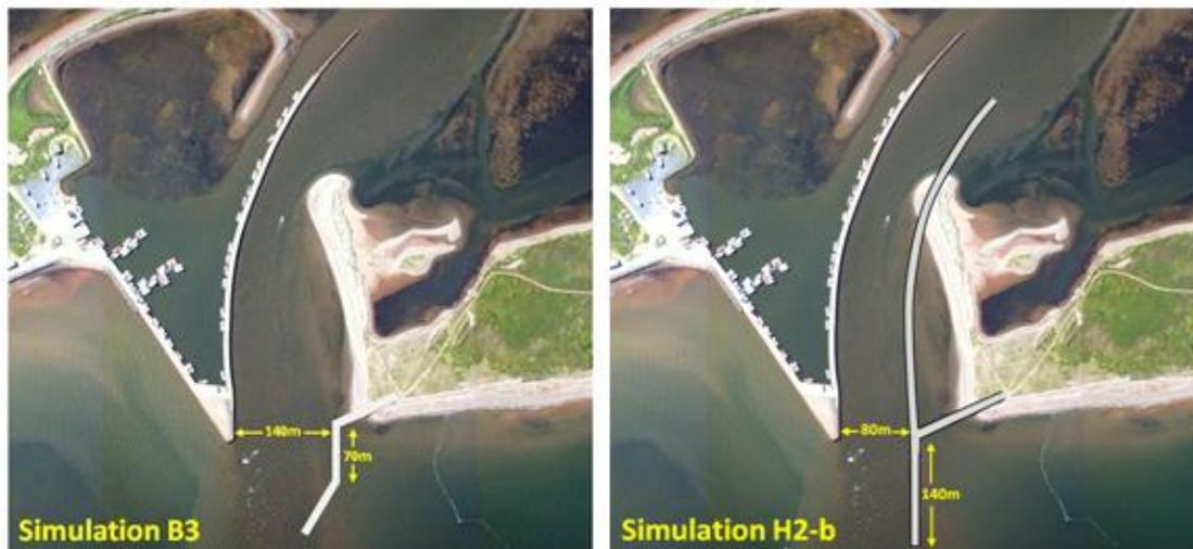
Figure 12. Examples of a new east jetty concept (left) and a parallel training wall culminating in a jetty (b) which were simulated using the calibrated numerical model.
