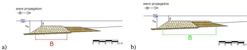
**Figure 8. Sections of the submerged barrier at the toe of the perched beach and indication of the mean equivalent width  $B$  considered for the comparisons with Gonzalez et al. (1999). a) original configuration; b) modified configuration.**
