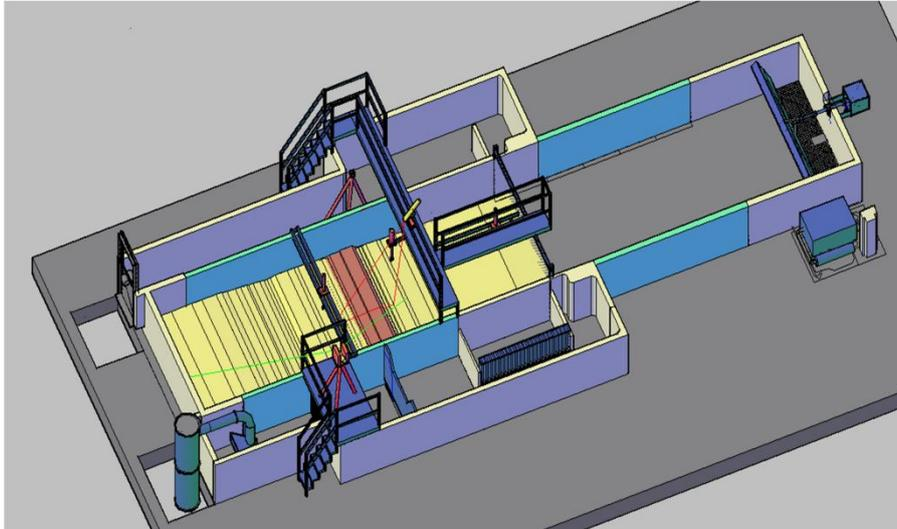
Figure 4. Experimental wave tank and location of the physical model of the perched beach nourishment (the barrier is in red), and of the measurement instruments.
