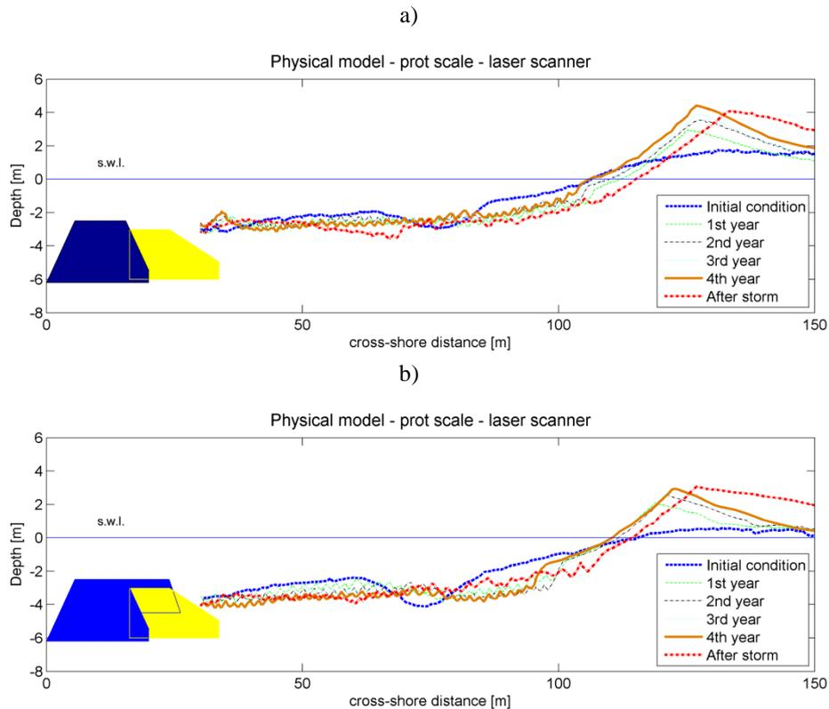
**Figure 7. Evolution of the beach profile measured at the end of several series of accretive waves (1<sup>st</sup> year, 2<sup>nd</sup> year, 3<sup>rd</sup> year and 4<sup>th</sup> year, each year is made up by about 12500 waves) followed by a series of erosive wave (small storm having about 2 years return period). a) original configuration; b) modified configuration. Measurements are reported at prototype scale.**
