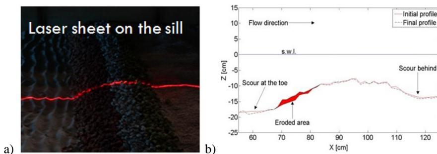
Figure 5. 2D computer vision system for recovery the damage to the submerged barrier and the scour depth close to it. a) formation of the image; b) interpretation of the image to measure the eroded area and the scour depth in front and behind the sill.
