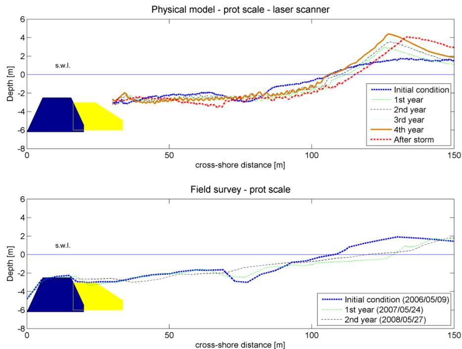
**Figure 11. Comparison of the beach profile evolution with field data. Top panel: beach profiles measured during the present experimental campaign; bottom panel: beach profile measured during field bathymetric survey.**
