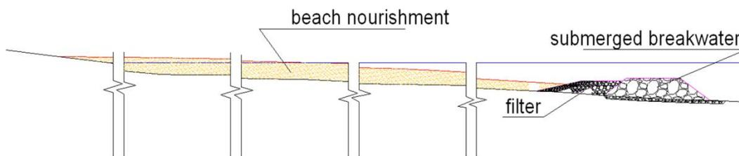
Figure 2. Design section of the beach nourishment intervention at the site of Belvedere Marittimo (Italy). The perched beach is protected by a submerged breakwater coupled with a filter system behind of the structure.
