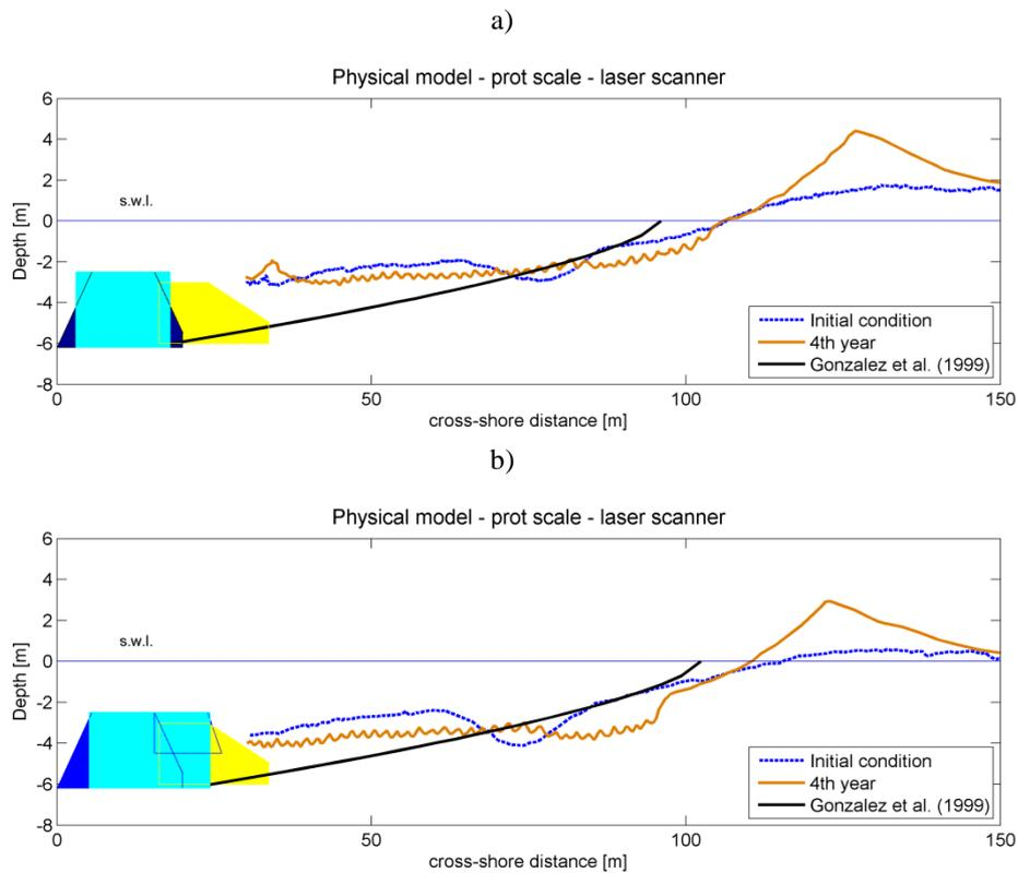
Figure 10. Comparison between the beach profiles measured and calculated by using the analytical model of Gonzalez et al. (1999) at prototype scale. The initial beach profile in blue is reported as a reference condition. The blue structure is the rubble mound sill, the yellow area represents the filter, the cyan region is the equivalent impermeable rectangular barrier considered in the application of the analytical model. a) original configuration; b) modified configuration.
