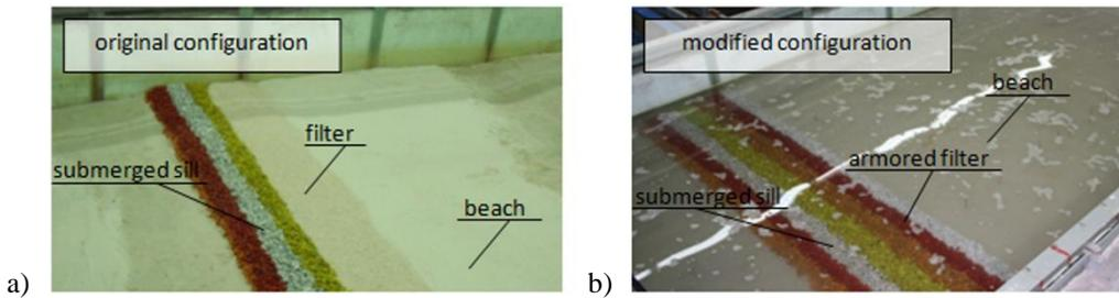
Figure 6. Investigated configurations of the perched beach nourishment: a) original configuration; b) modified configuration (where the filter has been covered with a layer of elements similar to those of the submerged sill).
