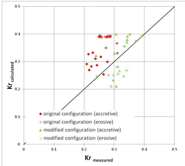
Figure 9. Comparison between the reflection coefficients measured and calculated by using the analytical model of Gonzalez et al. (1999).
