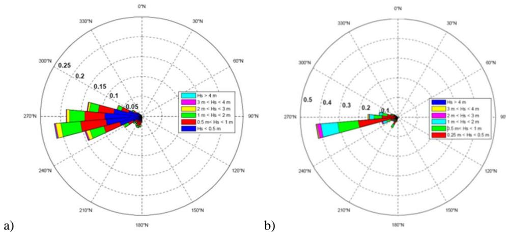
Figure 3. Directional distribution of significant wave height at the site of interest. a) Frequency of significant wave height in deep waters. b) Frequency of significant wave height at closure depth ( $h=7.2$  m).
