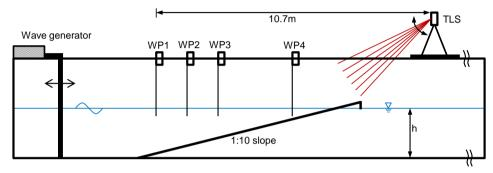
Figure 1 Diagram illustrating the experiment setup. The TLS is mounted above the wave flume to increase the visible water surface.
