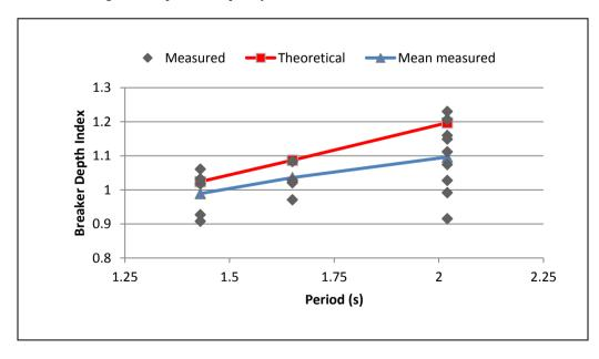
Figure 5 Breaker height index comparison
