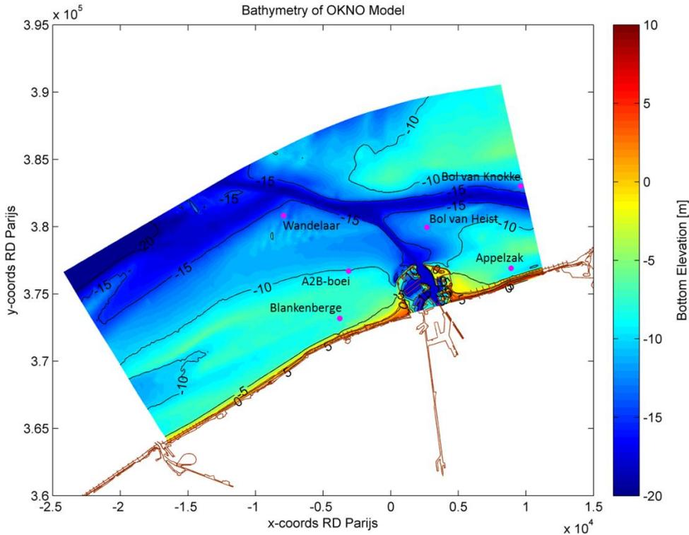
Figure 3 : Bathymetry of the Delft3D OKNO model, elevation in m NAP (equivalent to MSL).
