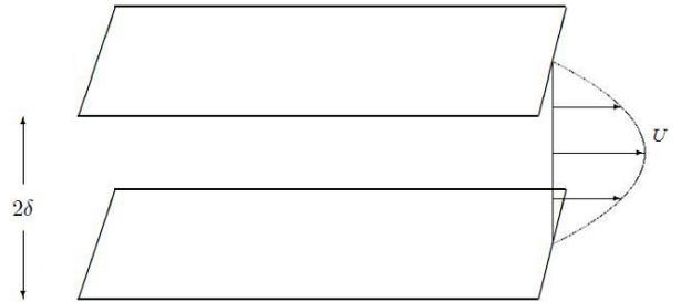
Figure 2. Test case: steady fully developed plane channel flow with smooth walls
