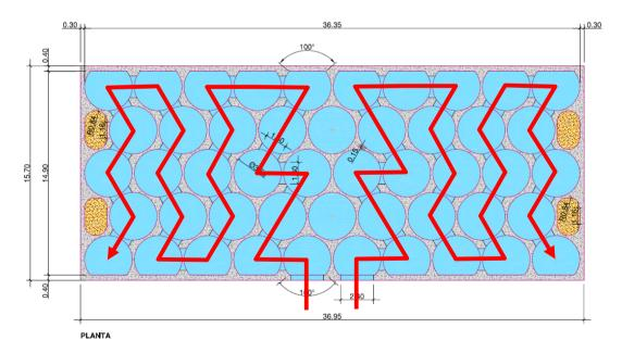
Figure 3. General view of the antireflective cyes-R caisson with two circuits of 23 cells each.
