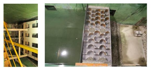
Figure 6. Absence of water leakages: a) wave paddle with interior face completely dry (left), b) model of the *cyes-R* with water on the left and dry (right).
