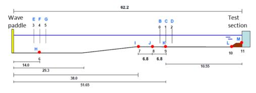
Figure 7. Experimental sketch. Vertical lines = resistance wave gauges. Red dots = ultrasound wave gauges.
