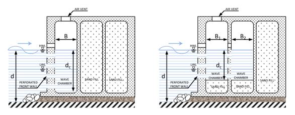
Figure 1. Jarlan-type structure with a) one chamber (left), b) two chambers (right).
