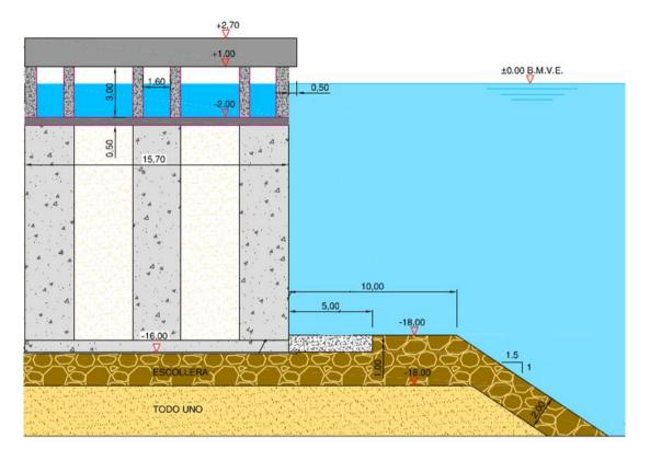
Figure 2. Cross section of the antireflective cyes-R caisson designed for 60 s < T < 200 s.
