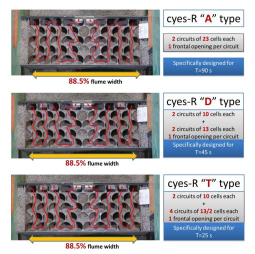
Figure 5. Typologies tested for the antireflective *cyes-R* caisson.
