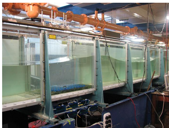
Figure 3. Waves running over the rough bed. Pressure sensors housed in boxes below.
