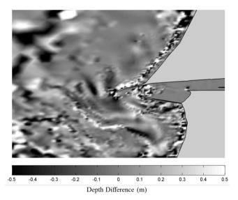
Figure 13. Depth difference between simulated bathymetries (Present - Future).
