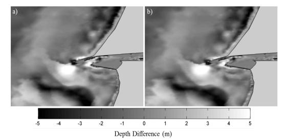
Figure 12. Difference between the computed final and initial bathymetries (meters) for a 1 year simulation considering the a) present and b) future wave regimes. Negative (positive) values represent erosion (accretion).
