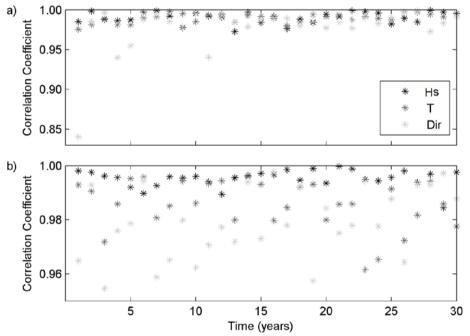
Figure 5. Correlation coefficient of wave height ( $H_s$ ), wave period (7) and wave direction (*Dir*) between each year and 30 years for: a) Present climate; b) Future climate.
