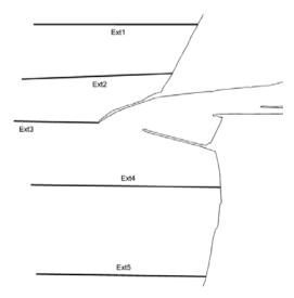
Figure 4. Sections location where transport of sediments is computed (Ext1 to Ext5). The sections were defined in order to be coincident with variations in the lagoon inlet bathymetry or geometry.
