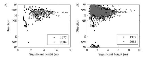
Figure 8. Wave direction in function of significant wave height: a) 60 days runs; b) one year runs.
