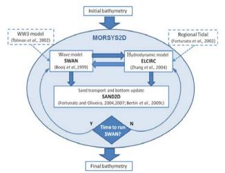
Figure 2. Schematic diagram of the MORSYS2D morphodynamic model system.
