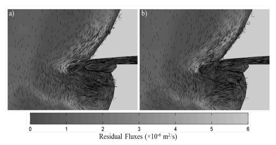
Figure 9. Residual sediment flux (m<sup>2</sup>/s) for simulations considering the a) present and b) future wave climate.
