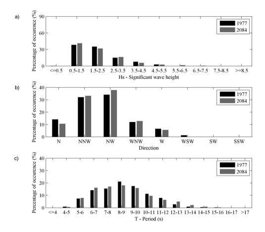
Figure 7. Annual distributions (%) of: a) significant wave height; b) wave direction; c) wave period.
