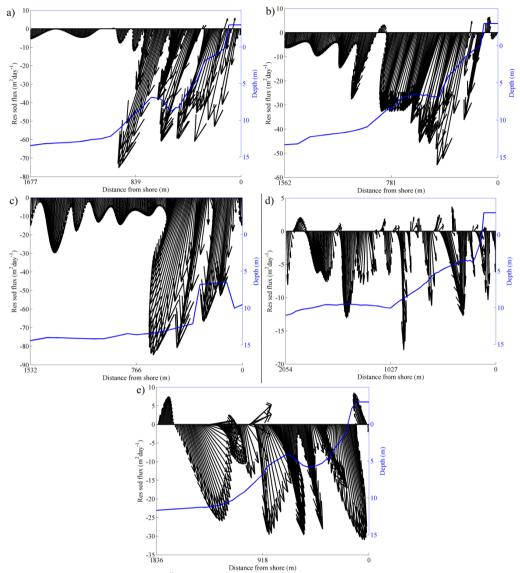
Figure 11. Residual sediment flux ( $m^2/day$ ) for the sections located at the offshore area of the inlet a) Ext1, b) Ext2, c) Ext3, d) Ext4 and e) Ext5, for simulations considering the present wave climate. The section depth is illustrated by the solid line and by the right axis of the subfigures.
