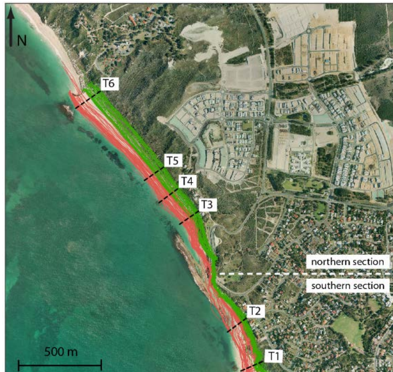
Figure 4. Vegetation lines (green) and instantaneous shorelines (orange) extracted from aerial photographs from 1971–2009, and transects where beach width was extracted (photo source: Landgate).
