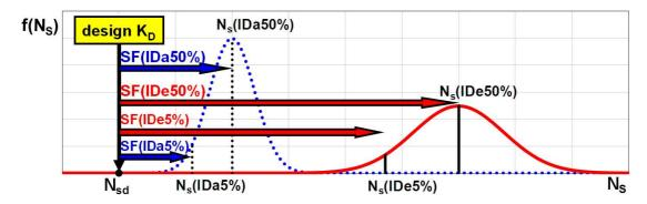
Figure 3. Schematic representation of design stability number (N<sub>sd</sub>) and Safety Factors to IDa and IDe.
