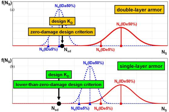
Figure 4. Schematic representation of damage criteria for (a) double-layer and (b) single-layer armors.
