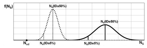
Figure 2. N<sub>sd</sub> and scheme of N<sub>s</sub>(IDa) and N<sub>s</sub>(IDe) probability density functions.
