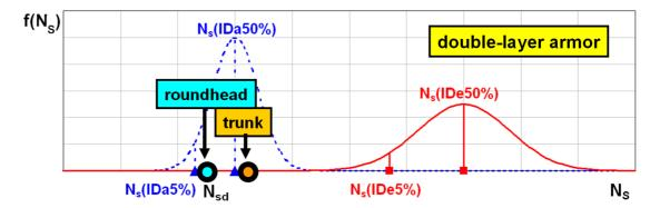
Figure 5. Schematic representation of design stability number (N<sub>sd</sub>) for roundheads compared to trunks.
