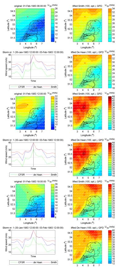
Figure 6. Original and uplifted wind fields for 01-02-1983 from 6 a.m. until 6 p.m, including wind speed time series at the reference location (4.375°E and 53.859°N). Optimal GPD estimates.
