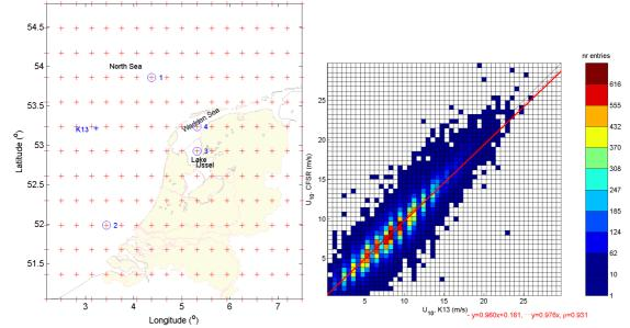
Figure 1. Left: Region covered by the considered CFSR data. Right: Comparison between CFSR and observed wind speeds.
