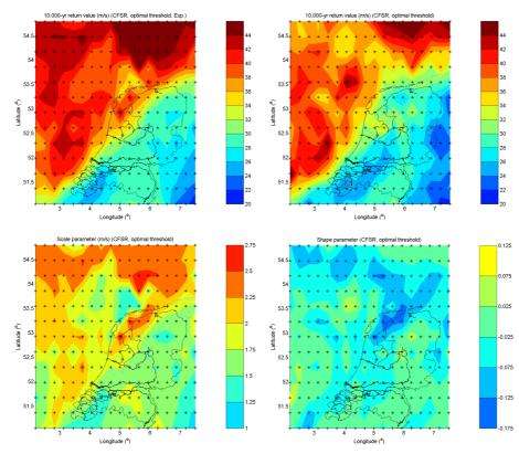
Figure 2. Estimates associated with a POT sample collected using the optimal threshold. Top panels: Local 10,000-yr return value estimates of the Exponential distribution (left) and the GPD (right). Bottom panels: Local GPD scale (left panel) and shape (right panel) parameter estimates
