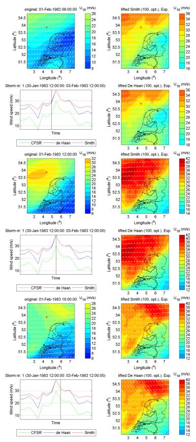
Figure 4. Original and uplifted wind fields for 01-02-1983 from 6 a.m. until 6 p.m, including wind speed time series at the reference location (4.375°E and 53.859N).
