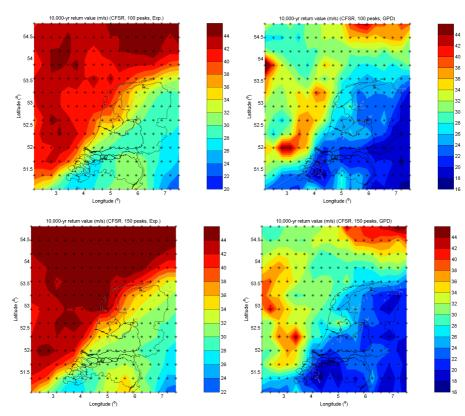
Figure 3. Top panels:Local exponential distribution (left) and GPD (right) 10,000-yr return value estimates associated with a POT sample with size 100 panel estimates. Bottom panels: Local exponential distribution (left) and GPD (right) 10,000-yr return value estimates associated with a POT sample with size 150.
