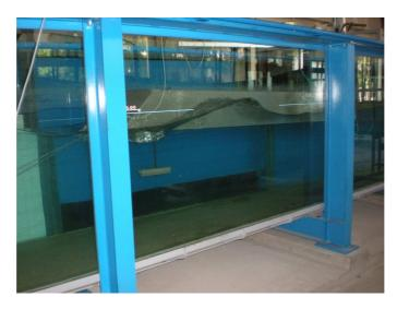
Figure 8. The SeaBreath tested in the wave flume at Padova University.
