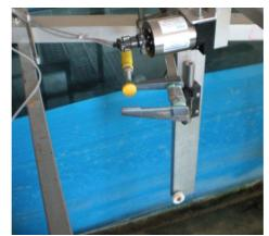
Figure 11. Displacement meter for surge movements: it is a rheometer with a wire mounted vertically and redirected in the horizontal direction by a lower wheel.
