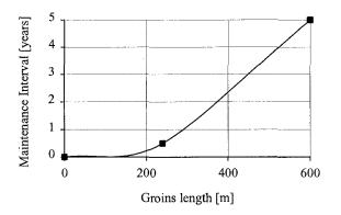
Figure 11. Groins length versus maintenance interval for Navia inlet (Functionality: 90%)
