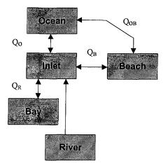
Figure 7. Morphological units of a tidal inlet.
