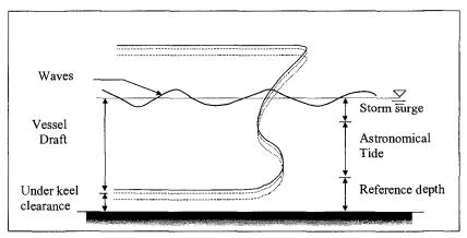
Figure 4. Real and required channel depth definition.
