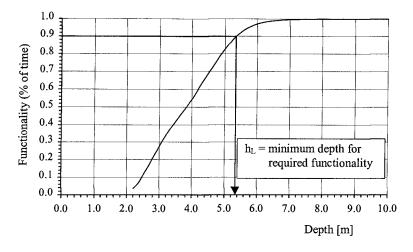
Figure 5. Functionality versus channel depth for the design vessel.
