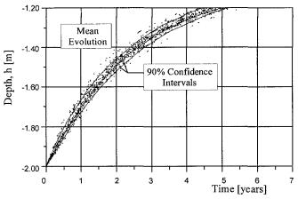
Figure 10. Time mean evolution for the short groin scenario (240 m) and 90% confidence intervals.
