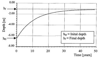
Figure 8. Time mean evolution for the long groin scenario (600 m).
