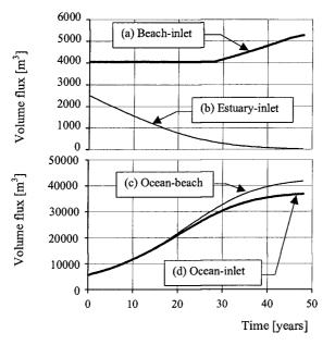
Figure 9. Sediment fluxes for the long groin scenario. Beach-inlet flux (a), estuary-inlet flux (b), ocean-beach flux (c) and ocean-inlet flux (d).
