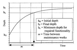
Figure 6. Time evolution example of channel depth.
