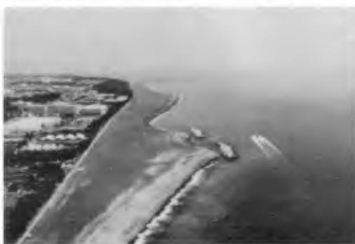
**Photo.6** The shoreline around detached breakwaters III. In this area, the foreshore is still fairly wide.
