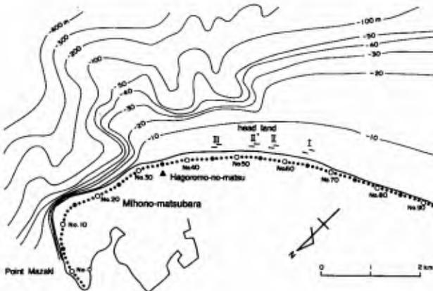
Fig.3 Detailed sea bottom contours off Shimizu coast and alignment of measuring lines.
