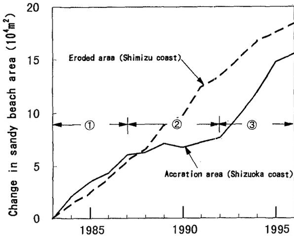
Fig.5 Change with time in eroded and accretion areas along Shizuoka and Shimizu coasts.
