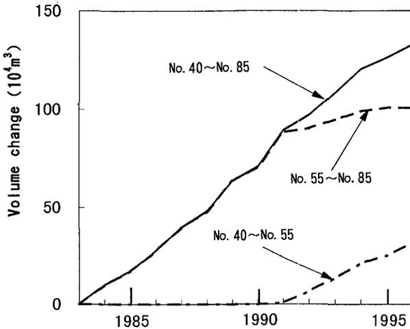
**Fig.6** Change in sand volume with time in the regions between No.55 and No.85, and between No.44 and No.55 along the Shimizu coast.
