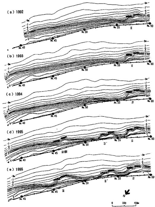
**Fig.11** Sea bottom changes around the detached breakwaters between March 1992 and March 1996.
