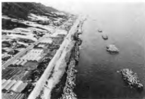
**Photo.3** Coastline protected by a continuous seawall, concrete armor units and a number of detached breakwaters further north of the location shown in Photograph 2 on the Shimizu coast.
