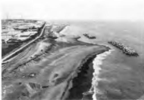
**Photo.4** The shoreline around detached breakwaters I. A couple of detached breakwaters were built alongshore. The offshore distance of the detached breakwater downcoast is close to the original shoreline. Large cusped foreland was formed behind the upcoast detached breakwater.
