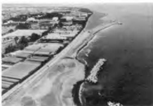
**Photo.5** The shoreline downcoast of detached breakwaters II'. Downcoast erosion was so severe that beach nourishment is being conducted, as shown in the photograph of the most severely eroded location.
