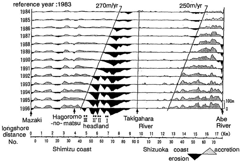
**Fig.4** Shoreline changes along the Shizuoka and Shimizu coasts showing the propagation of erosion and accretion waves. The propagation velocities of erosion and accretion waves are around 270m/yr and 250m/yr, respectively.
