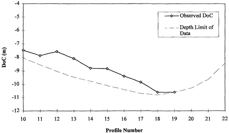
Figure 3. Observed longshore variation in depth of closure from 1965 to 1990, calculated using the SDDC method.
