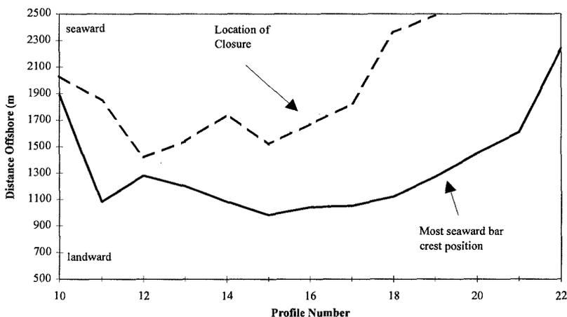
Figure 9. Location of closure (SDDC) in the JARKUS data and the most seaward bar crest position for the period 1965-1995.
