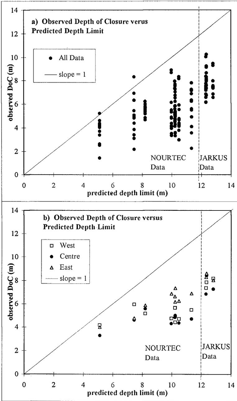
Figure 8. Observed depths of closure versus predicted depth limit of active profile. a) shows all data, b) shows average values for the western, central and eastern sections of the study area.
