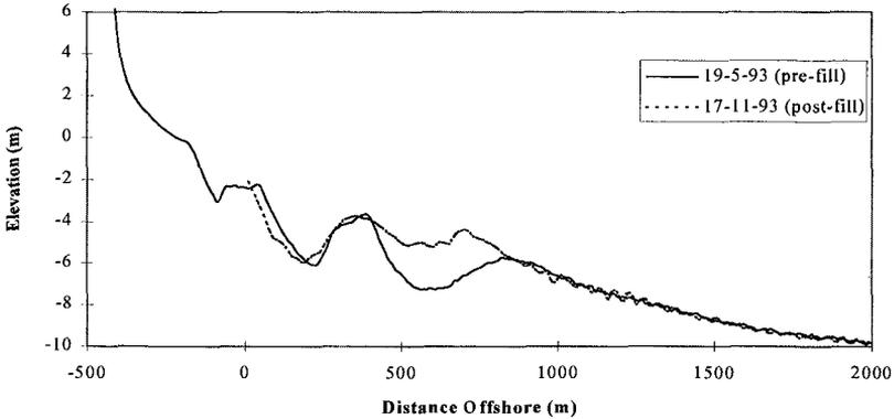
Figure 2. The fill material was placed between the middle and outer bars of a triple barred system.
