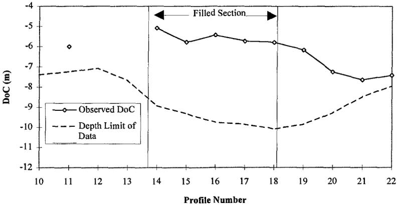
Figure 6. Observed longshore variation in depth of closure determined using the SDDC technique for the post-fill period (17th November 1993 to 13th December 1995).
