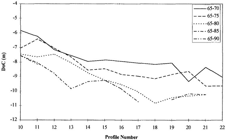
Figure 5. Observed depth of closure determined using a fixed criteria depth change criterion of 50 cm for an expanding time window for 5 to 25 years (relative to 1965).
