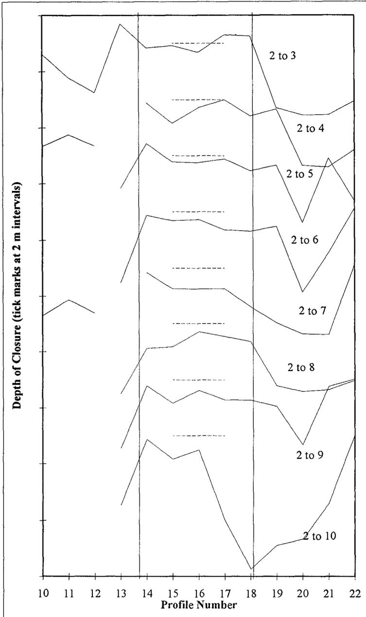
Figure 7. Time-expanding envelope, post-fill depths of closure. Intervals refer to survey numbers shown in Table 1. Each interval is offset by 2 m, and the dashed line indicates -5 m on each transect. The vertical lines mark the fill boundaries.
