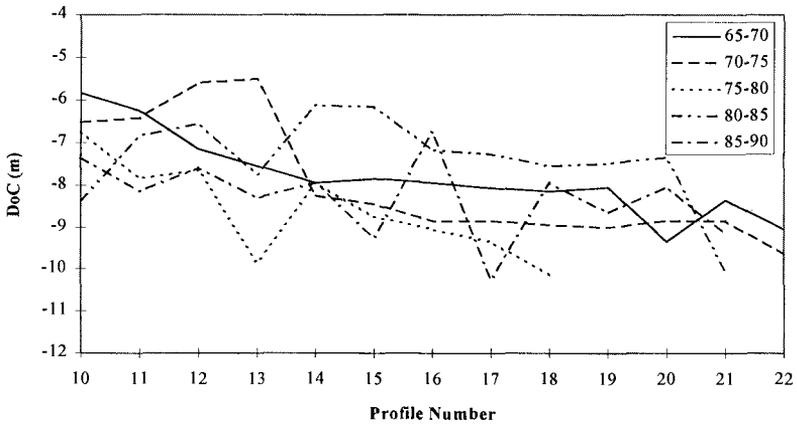
Figure 4. Observed depths of closure determined using a fixed criteria depth change criterion of 50 cm for five-year time intervals.
