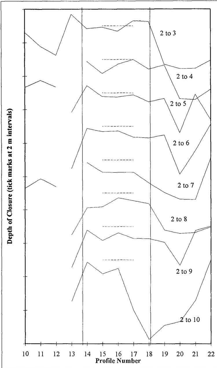
Figure 7. Time-expanding envelope, post-fill depths of closure. Intervals refer to survey numbers shown in Table 1. Each interval is offset by 2 m, and the dashed line indicates -5 m on each transect. The vertical lines mark the fill boundaries.
