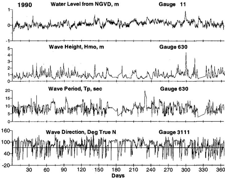
Figure 3: Observed wave and water level parameters at Duck, NC, in 1990
