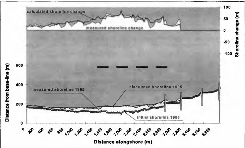
**Figure 12. Ras-El-Bar model verification and final results**
