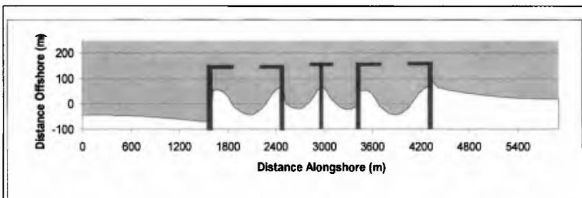
**Figure 3a. Shoreline response to coastal structures**
