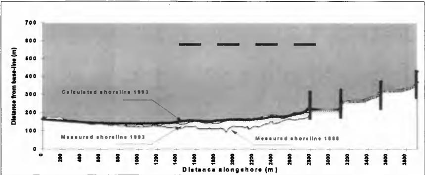
**Figure 11. Ras-El-Bar model calibration results**
