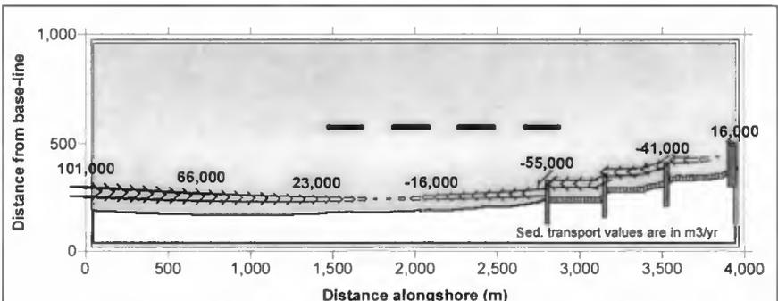
**Figure 14. Net annual longshore transport rates along the modeled area**
