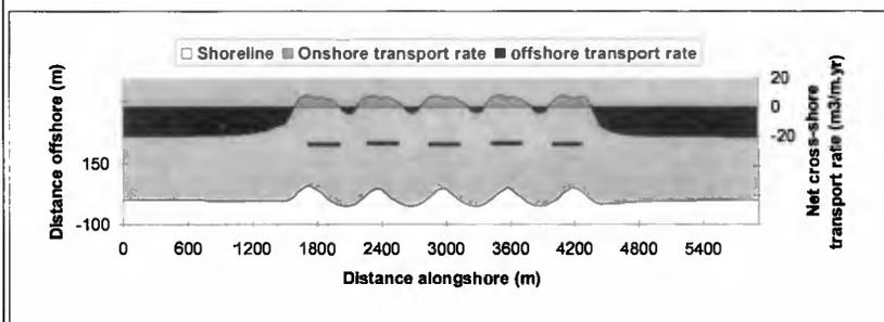
**Figure 3c. Shoreline response and cross-shore transport pattern near breakwaters**
