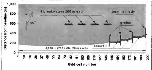
Figure 10. Schematic diagram of the modeled region
