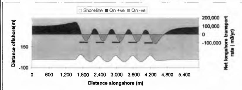
**Figure 3b. Shoreline response and longshore transport patterns near breakwaters**
