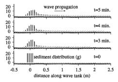
Figure 5 Movement of particle(fine sand) above distorted ripple train. Experimental condition : T=1.5s, H=0.08m, h=0.35m.
