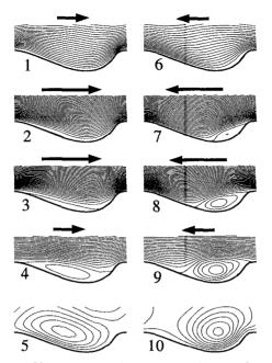
Figure 6 Variation of  $\psi$  during one oscillatory flow cycle
