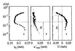
Figure 3 Velocity distribution above ripple crest.  $u_a$ : wave velocity amplitude,  $u'_{rms}$ : turbulent intensity, U: steady flow. Experimental condition: T=1.5s, H=0.08m, h=0.35m.
