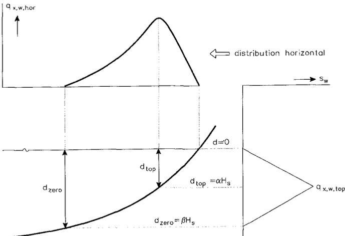
Figure 2: Schematic of wave-induced longshore transport
