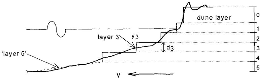
Figure 1: Layer schematization used in the model
