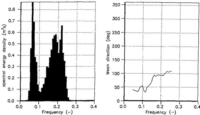
*Fig. 3 Typical wave spectrum at Pecém. Two distinct peaks can be observed with frequencies of approximately 0.08 and 0.12 s<sup>-1</sup> representing swell and wind waves (sea) respectively. The wave directions of the two dominant wave components are varying from approximately 30° N for the swell to approximately 120° N for the sea waves.*
