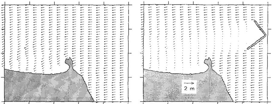
Fig. 5 Simulated wave field (Sea).  $H_s=1.75\text{m}$ ,  $T_p=7\text{s}$ ,  $MWD=82.5^\circ$
