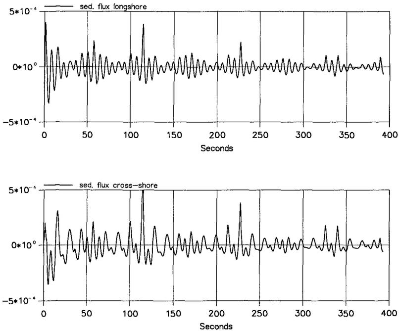
Fig. 11 Instantaneous sediment flux due to different wave groups.
