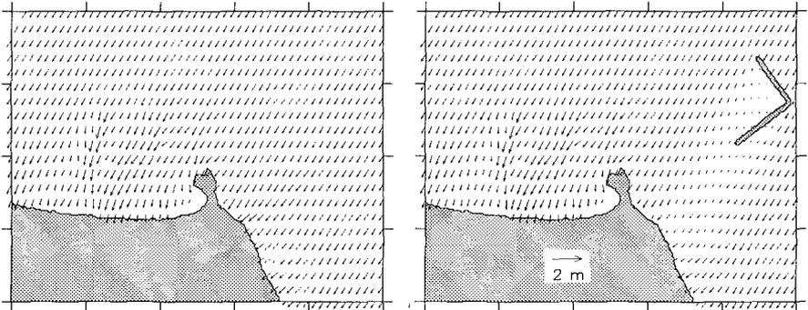
Fig. 6 Simulated wave field (Swell).  $H_s=0.5m$ ,  $T_p=14s$ ,  $MWD=30^\circ$
