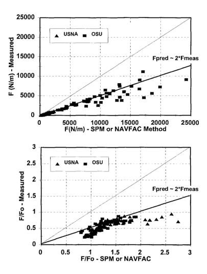
Figure 2. Comparison of measured forces to forces predicted using SPM or DM26.2 design method, for regular waves.
