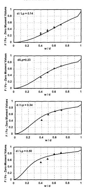
Figures 5. Comparisons of measured and predicted wave forces for irregular waves, for selected values of relative depth  $d/L_p$ .
