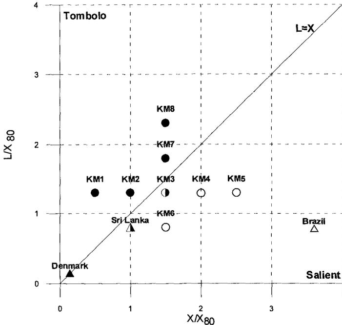
Figure 6. Calculated morphological response as a function of the length and location of the detached breakwater. Triangles: field data. Circles: model results. Open symbols: salient. Filled symbols: tombolo.
