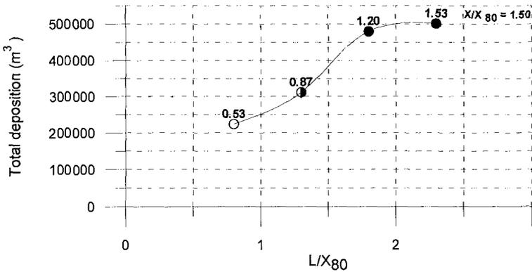
Figure 8 Influence of structure length on the amount of sediment deposited on the initial bathymetry. All breakwaters have  $X = 360\text{m}$ . Figures on the plot correspond to values of  $L/X$ . Symbols as in Fig 6.
