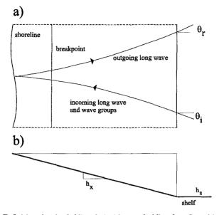
Figure 1: Definition sketch of obliquely-incident and obliquely-reflected infragravity waves. a) plan view; b) cross-section.
