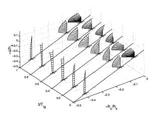
Figure 3: Infragravity wave profiles for three locations  $(h_o/h_s = 0.42, 0.17 \text{ and } 0.07)$ and for five time instances of the infragravity wave period. The breakpoint is located at  $h_o/h_s = 0.3$ .
