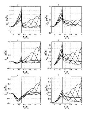
Figure 5: Magnitude of B and D coefficients vs. cross-shore distance  $h_o/h_s$  for five intervals per IG wave period: (a)  $B_{xx}$ . (b)  $D_{xx}$ . (c)  $B_{xy}$ . (d)  $D_{xy}$ . (e)  $B_{yy}$ . (f)  $D_{yy}$ . The stillwater shoreline is located at  $h_o/h_s = 0$  and the breakpoint at  $h_o/h_s = 0.3$ . Also shown as the thick solid line is the magitude of the terms for the case of no groupiness  $\delta = 0$ .
