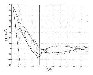
Figure 2: Envelope of the surface elevation of an IG wave vs. cross-shore distance: linear analytical solution by Schäffer & Svendsen (1988) (dash-dot line), SHORE-CIRC without Q-3D terms (dashed line), and SHORECIRC with Q-3D terms (solid line). The breakpoint is located at  $h_o/h_s = 0.3$ .
