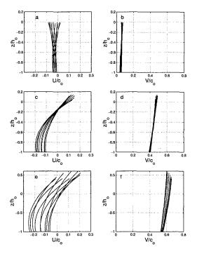
Figure 4: IG wave particle velocities in the cross-shore and longshore direction normalized by the longwave celerity  $c_o$  vs. normalized depth for ten intervals per IG wave period: (a) Cross-shore velocity U at  $h_o/h_s = 0.42$ . (b) Longshore velocity V at  $h_o/h_s = 0.42$ . (c) U at  $h_o/h_s = 0.17$ . (d) V at  $h_o/h_s = 0.17$ . (e) U at  $h_o/h_s = 0.07$ . (f) V at  $h_o/h_s = 0.07$ .
