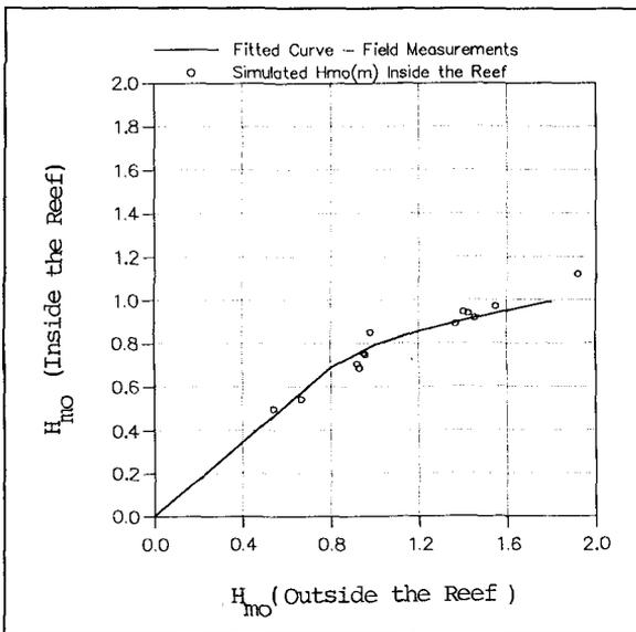
**Figure 2. Verification of Wave Transmission Over the Secondary Reef**
