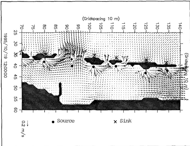
Figure 5. Simulation of Wave Overtopping Currents Behind the Secondary Reef
