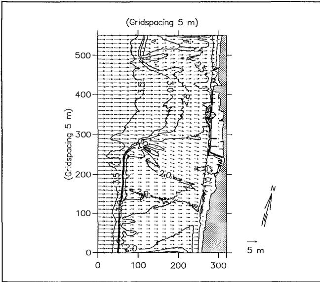
**Figure 3. Simulation of 100 Year Return Period Wave at 0.0 m MSL**
