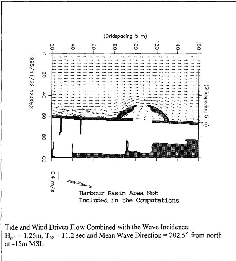
**Figure 8. A Simulated Hydrodynamic Scenario for Sediment Transport Computations**
