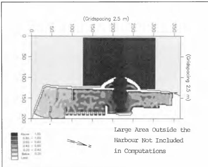
Figure 7. Simulated Significant Wave Heights Exceeded 1 Week per Year
