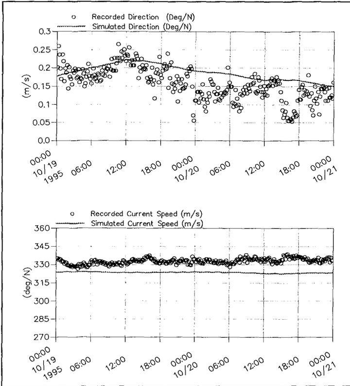
**Figure 6. Simulated and Recorded Currents Behind the Secondary Reef**
