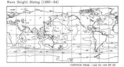
Fig.8 Increase of wave height during 10 years from 1985 to 1994. Contour lines show the total increase of wave height. Solid lines indicate positive values (increase) and dashed lines indicate negative values (decrease). The increase was obtained by fitting a linear regression curve to the monthly mean wave height.
