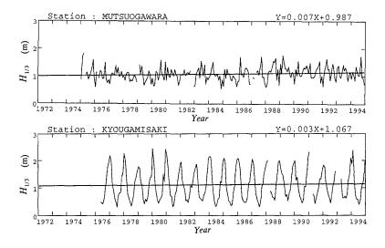
Fig.4 Time series of monthly mean wave height and the liner trend. (top figure; the Pacific coast, bottom figure; the Japan Sea coast)
