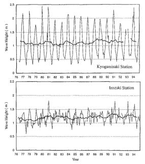
Fig.2 Annual variation of monthly mean wave height (thin line) and 12 months running mean (thick line). (top figure; the Japan Sea coast, bottom figure; the Pacific coast)
