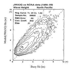
Fig.7 Scatter plot of modeled and measured significant wave height for NOAA buoys in the North Pacific.
