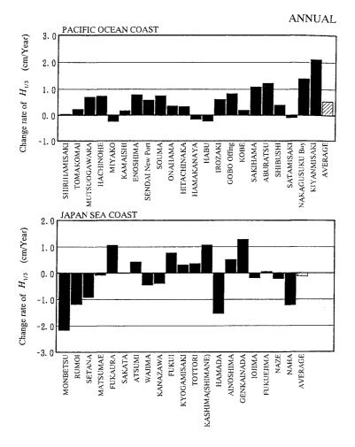
Fig.5 Long-term change rate (cm/year) of the significant wave height. (top figure; the Pacific coast, bottom figure; the Japan Sea coast)
